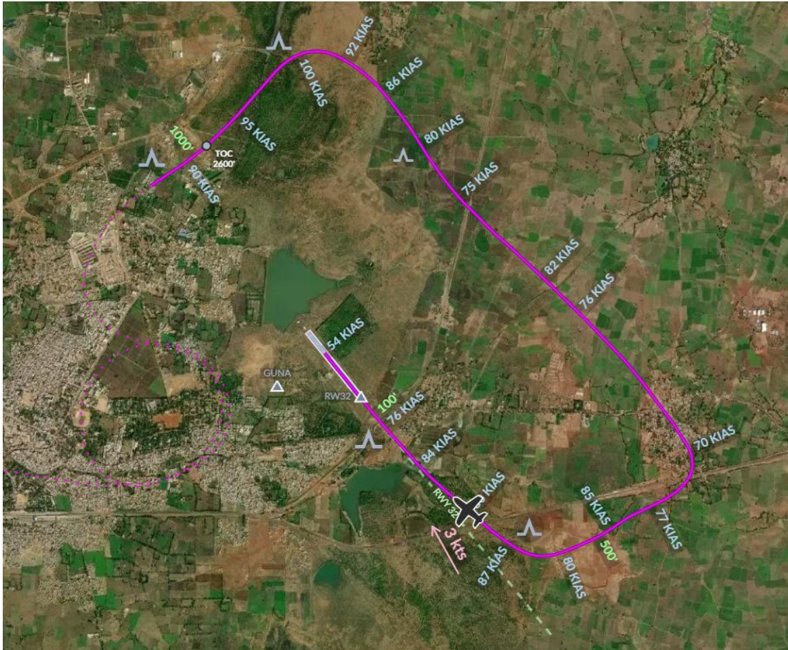
Figure 16. Aircraft speed along circuit
