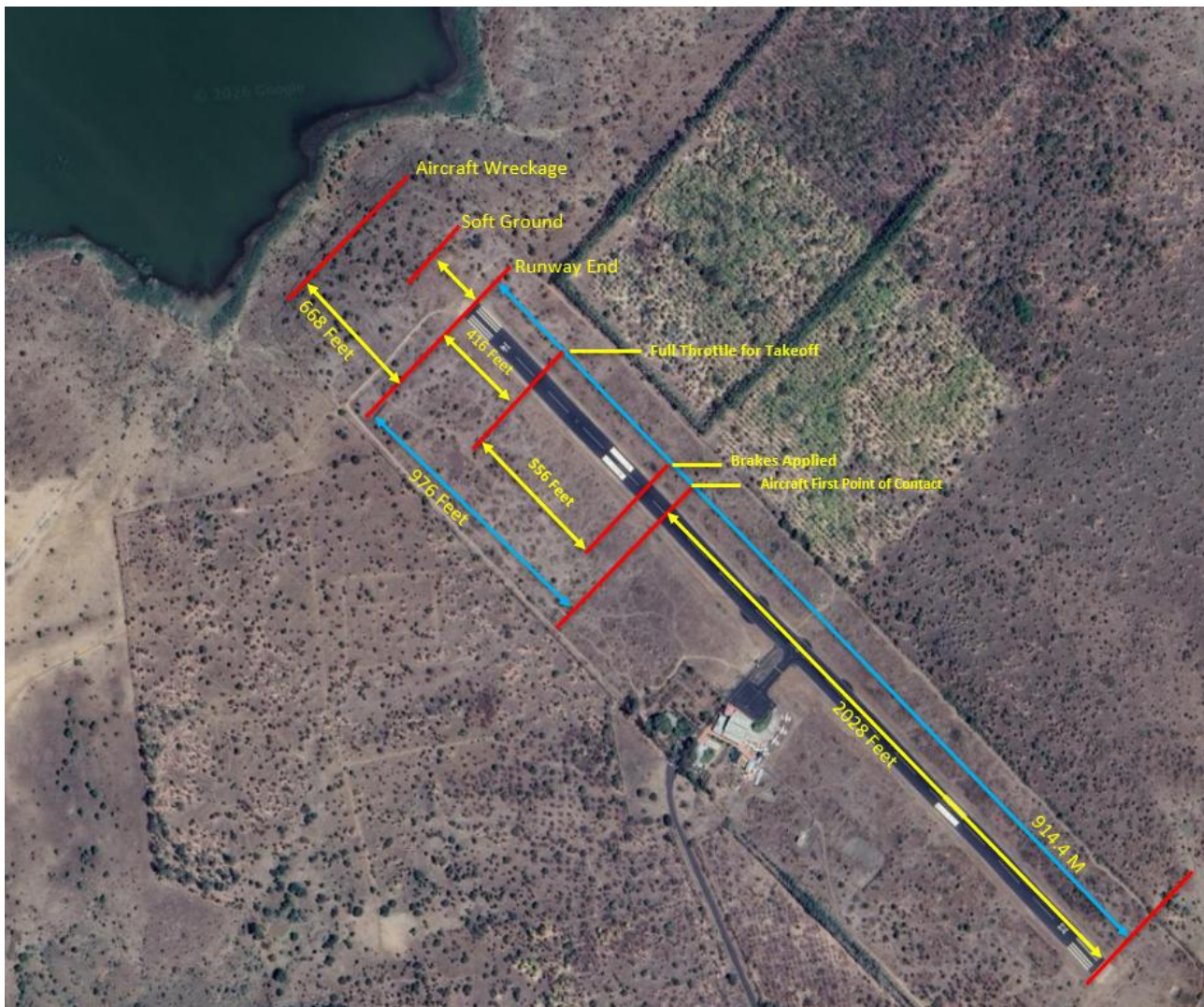
Figure 7. Projection of aircraft distance at different locations along the runway
